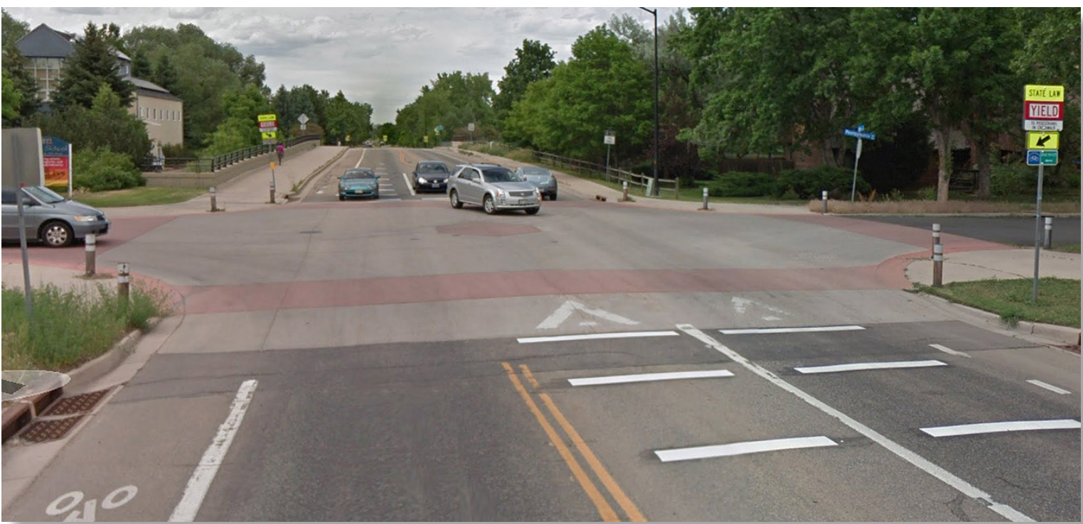
Figure D: Raised intersection; Photo source: space4cyclingbne.com
